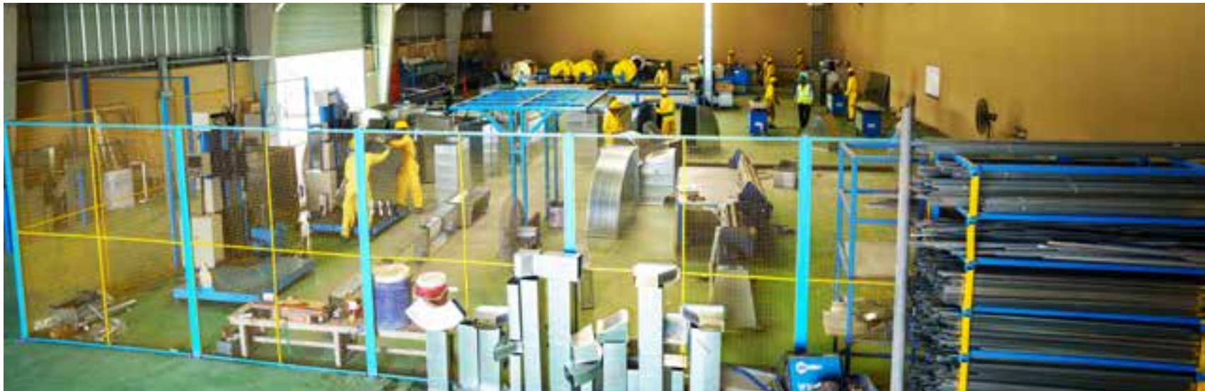
This 1,500 sq metres of covered facility is equipped with autoline and plasma cutter for duct manufacturing for AC ducting, duct connectors, flanges and pre-insulated ducting volume dampers
