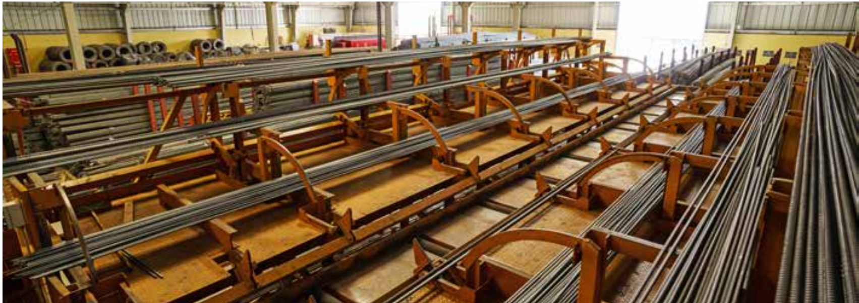
3,800 sq metres of covered facility, houses shear line, robot bender and automatic stirrup bending machines for carrying out structural works – 30,000 tonnes per annum.
